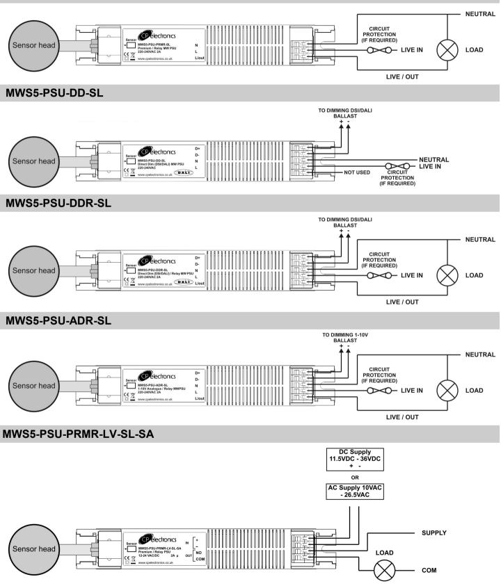
Note. Due to the proximity to other terminals ,the low voltage supply (AC or DC) cannot be SELV if the output connections are mains (ie, non SELV).
