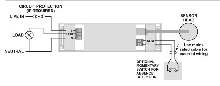
MWS5-DD, MWS5-AD Dimming - switch Option A
